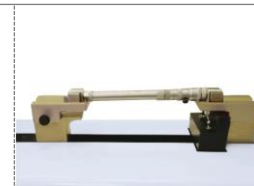
zero setting and calibration of tubular inside micrometers
