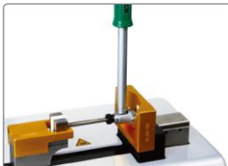
zero setting and calibration of bore gauges
