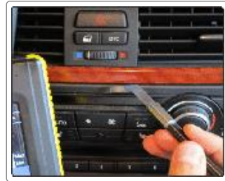
Measuring gaps on the car dashboard
