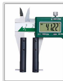
spherical points for groove diameter (inside hole) measurement
