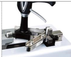
zero setting and calibration of three-point internal micrometers
