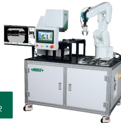
Automatic Quick Measurement System RBT-QM01
