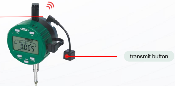
02 Transmitter Connecting to micrometer
