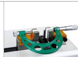
zero setting and calibration of micrometers
