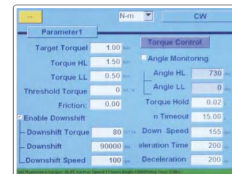
Interface of tightening parameter setting
